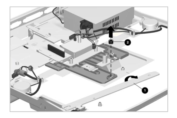
Figure 6-32. Removing the Docking Bar and Bushing
